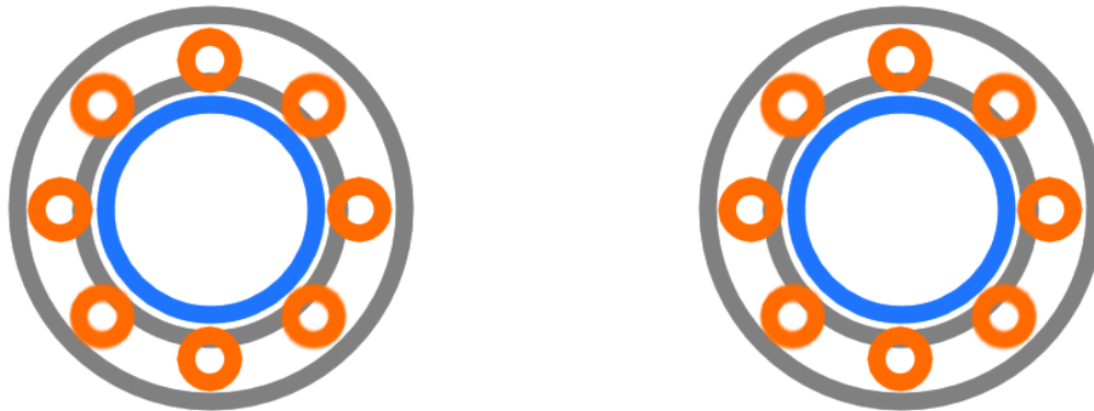
Figure 23: Round Linear Rail - Profile of a round linear rail. Gray is the linear bearings of the carriage. Orange is the ball bearings inside the linear bearings. Blue is the rail.
